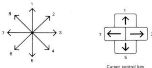
When the keyboard is selected by specifying 0 as f, integers 2, 4, 6, and 8 are returned when two cursor control keys are pressed at the same time, as shown below.
