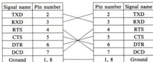
Use both units in the terminal mode. (Refer to the manual for the RS-232C interface.)
