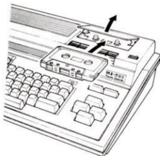
Close the cassette compartment cover by hand. Press the **C** key on the main keyboard. (Pressing the **M** key starts the monitor. See Chapter 8.) The screen display will change as follows:
