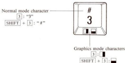
**In the normal mode:** when a character key is pressed, either the uppercase type for the letter marked on the keytop or the lower character on the keytop is input. When the character key is pressed together with the **SHIFT** key, either the lowercase type for the letter marked on the keytop or the upper character on the keytop is input.
