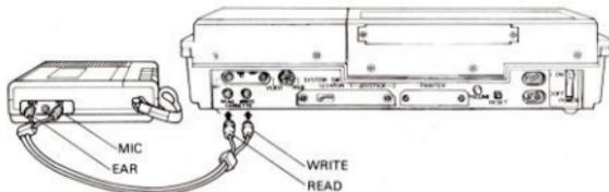
Note the following when using an **ordinary cassette tape recorder**.
